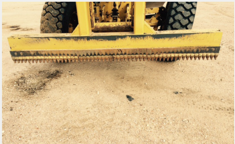
FIGURE 7: Scarifier with bullet teeth. (Pawnee County)
