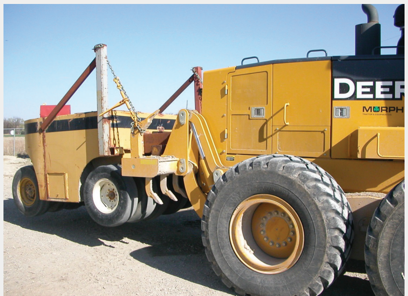
FIGURE 5: Roller mounted on grader. (Pleasant Twp. in Butler County)
