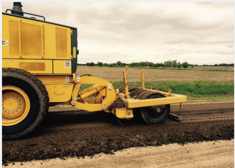
FIGURE 6: Roller on grader. (Pawnee County)
