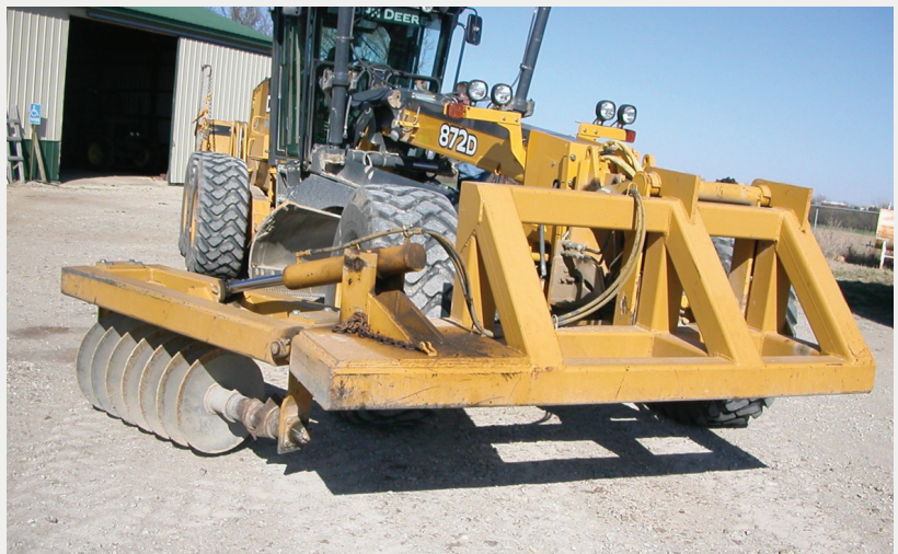
FIGURE 1: One-way disc for recovery of gravel and to break up sod. (Pleasant Twp in Butler County)
