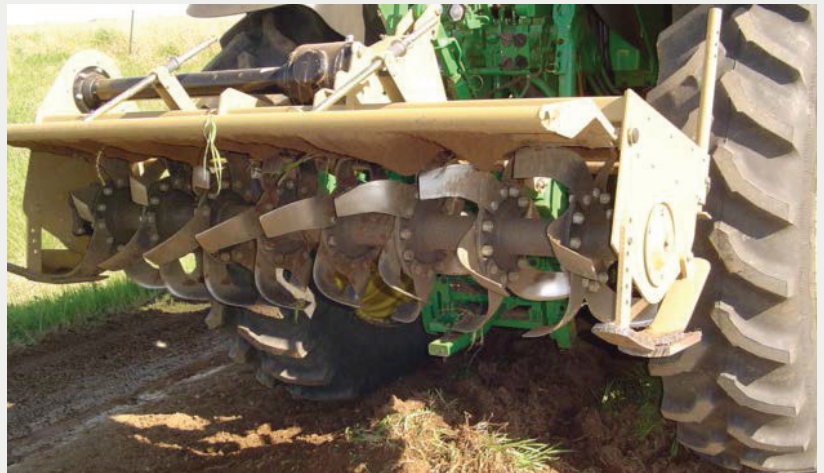
FIGURE 4: Tiller for breaking up sod in a windrow. (Gravel Roads Construction and Maintenance Guide)
