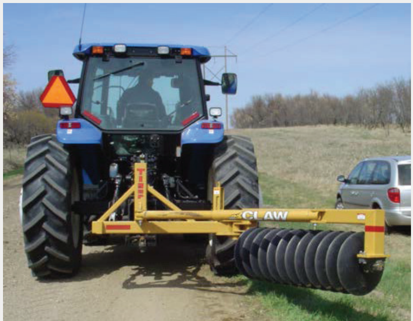
FIGURE 2: Tractor mounted one-way disc. (Gravel Roads Construction & Maintenance Guide)
