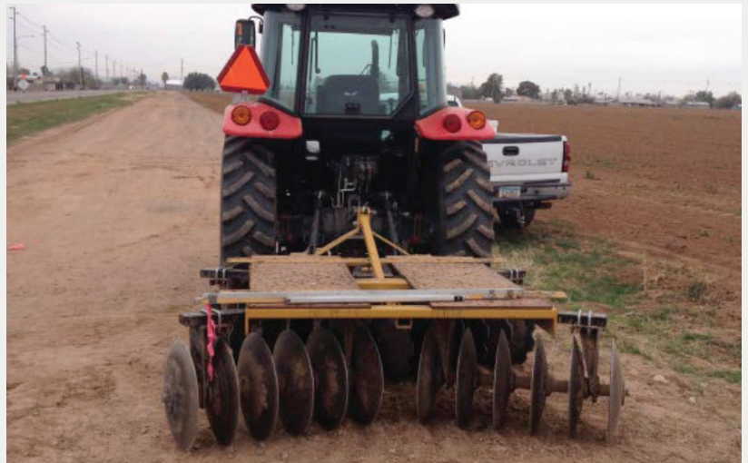
FIGURE 3: Farm disc can work for breaking up sod in windrow. (Gravel Roads Construction & Maintenance Guide)
